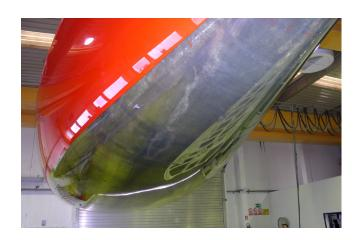
The slamming zone of the boat has been built a single skin composite in order to avoid shear failure of core material under the heavy loads. That area is additionally reinforced with layers of triaxial E-glass fabric.
